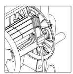
The high pressure washer comes in two models: A) with hook for storage of high pressure hose (14) - B) with a hose reel (13), where the hose is pushed into the reel and afterwards winded up.
